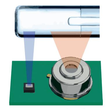
Figure 5: Infrared temperature sensor in both SMD and TO-can packages. Narrow FOV and optimum distance from the cartridge must be selected for accurate sensing.
